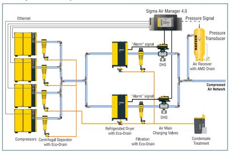
The second example shows a multiple compressor system with two parallel air treatment lines all controlled by a Sigma Air Manager (SAM) 4.0. A standard feature of the DHS is its ability to connect to a SAM 4.0. The SAM 4.0 can modify DHS 4.0 parameters and monitor for alarms. With optional inputs, the DHS can also close in case of a dryer failure.
