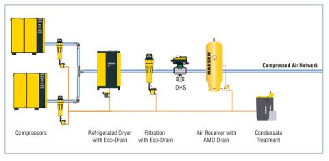
When the supply of air is the priority, the air main charging valve is set so that the default is "normally open". In case of power failure, the valve remains open, ensuring air supply. For systems which are shut down infrequently and have no leaks in the supply side piping, this field adjustable setting allows for any storage receiver after the air main charging valve to supplement air during start up conditions, further minimizing system exposure to high velocity air.
