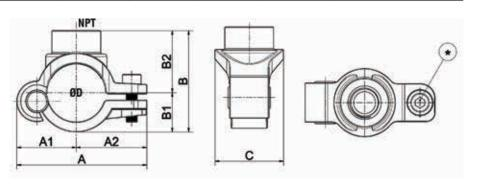
Note: Requires hole saw bit to drill pipe. 1/2" = 14 mm hole saw drill bit (ANK0043). 3/4" = 19 mm hole saw drill bit (ANK0143). 1" = 24 mm hole saw bit, includes Arbor and Pilot, (ANK0342). ANK0243 Drill arbor and pilot bit also required
