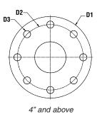
Includes 1 gasket and 4 bolts for 1" through 3" flange Includes 1 gasket and 8 bolts for 4" flange and above ANSI Class 150 Flange
