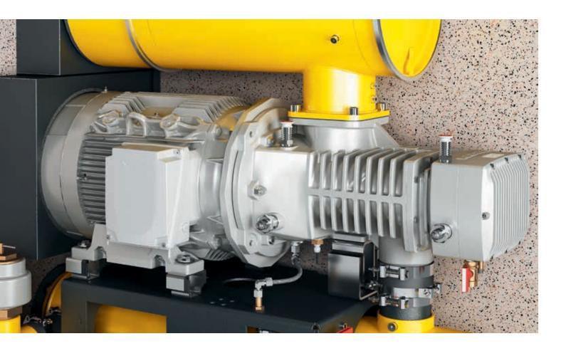
In CBS and DBS series blowers, power is transferred from the motor to the blower airend via an integrated gear drive. Following detailed testing in Kaeser's Research and Development Centers, this was found to be the most effective transmission solution for the speeds in this power size and machine class with regards to efficiency, dependability, and durability.
